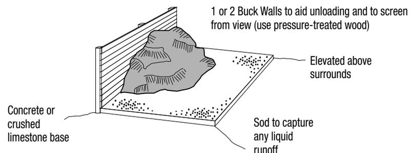
**Figure 7. Manure pad slope and drainage. Drain and gutter are recommended in all cases, especially if the manure stack will not be protected from rainfall. Leachate (effluent) must be directed to a storage tank and/or suitable method of disposal.**
